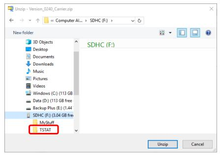
Verify that the files, including the BINF0405.hex file, have been extracted into the TSTAT folder of the MicroSD device. Note that the "USER" folder is where the photo and schedule files would be stored.
