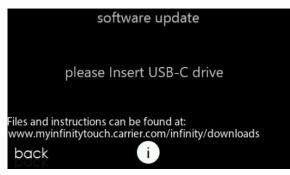
If the .bex file is stored properly on the USB-C drive, this screen will appear. If the screen says, "Please insert USB-C drive", remove the USB-C drive and re-insert. If it still does not show the screen, below, go back to the download part and retry.
